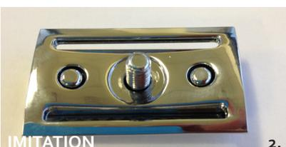
Edwin Jagger advises, the performance and ease of use of the imitation double edge safety razor heads similar to the sample we tested may be compromised by the issues we have highlighted above. Reduced blade support and insecure, inaccurate fittings may remove the possibility of a close, reliable and comfortable traditional wet shave.
